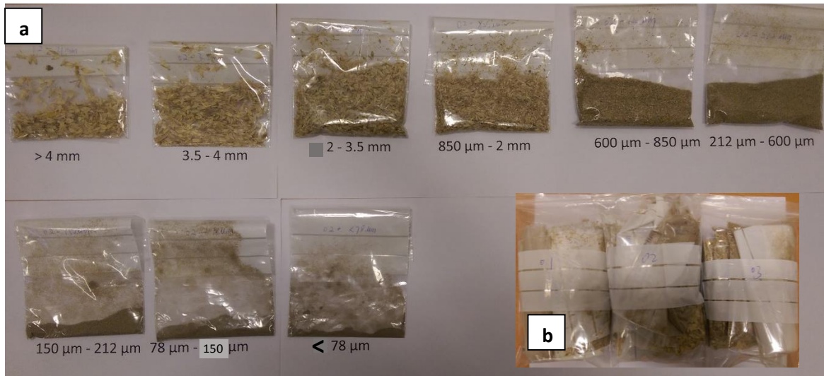
Fig. 2. Range of particle sizes in the grain dust as collected by the air cleaner (a). The 3 samples taken from the dust pile (b).
